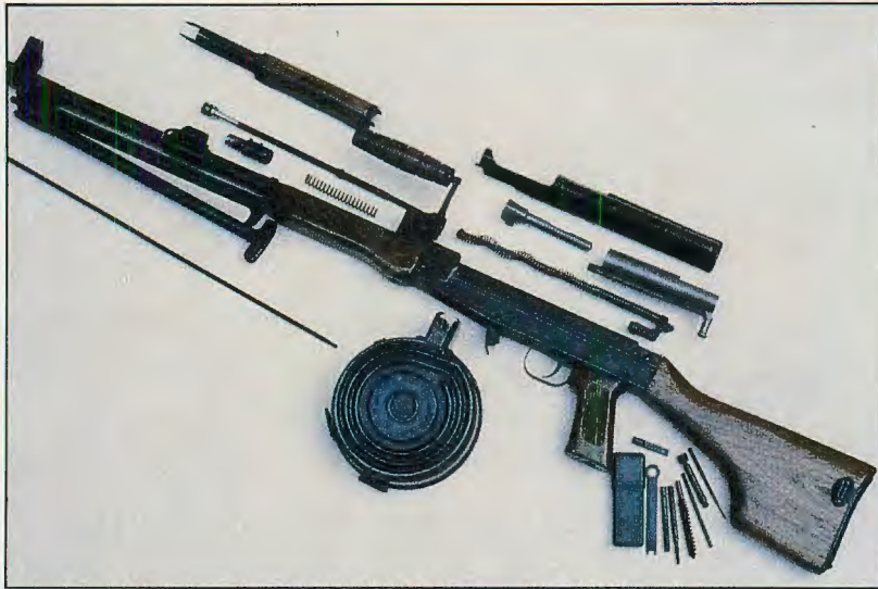
PRC Type 81 Squad Automatic Weapon (SAW), fieldstripped with 75-round drum and cleaning kit.
